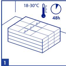
Installation must be performed between 18-30°C. Quick-Step Vinyl floors must be acclimatized in the room of installation between 18-30°C (64-86°F) for a period of at least 48 hours before installation. This floor- & roomtemperature needs to be maintained prior to, during and for at least 24 hours after the installation is completed.
