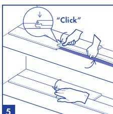
Click-it! Slightly lift the plank to be installed by holding your hand underneath about 25 cm from the end joint. Push the short side joint down gently with your thumb moving from the inner corner towards the outside until you hear/feel a click. Always check each short side joint (height differences and openings) before continuing. You can press down gently with your thumb on top of every short end joint to ensure good locking
